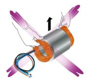
**Never**: lift a stator by its coil end turns only!
