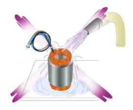
**Incorrect washing** of the stators: Do not wash stators with high pressure!
