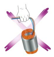
**Never**: lift, pull or tear a stator by its connection leads!
