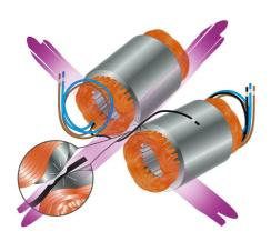
**Never:** squash power or sensor connection leads between laminated cores!
